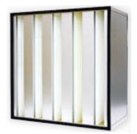
Airmax "SEMI HEPA PLUS-V" is designed for energy saving, and limited space. Every filters are individual test to ensure the quality to meet an efficiency of minimum ≥95‰n 0.3 micron particle size. Frame is made from either galvanized steel Aluminium. High capacity operation is achieved by designing additional media into the filter.
